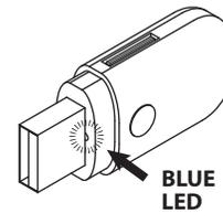
**Charge Battery:** Light blinks slowly. When fully charged, light remains on.
