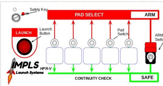
Insert the Safety Key and rotate to the ON position. The ARM switch should be SAFE and the paddle down to indicate Safe. Toggle the Pad Switches toward **CONTINUITY CHECK**. If it beeps then you are ready for operation.
