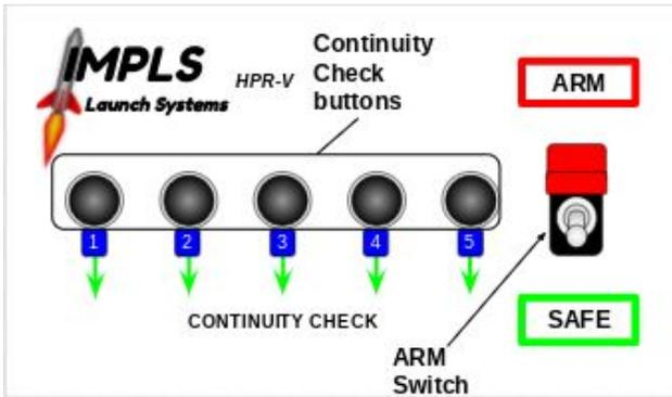
At this time the Arm switch should be set to safe, and the red paddle in the down position to indicate Safe. Distribute the launch leads to the launch pad positions.
