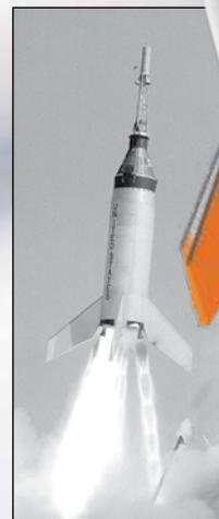
The Little Joe I booster was the first rocket designed solely for manned spacecraft qualifications and to measure critical parameters in flight.
