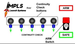
At this time the Arm switch should be set to safe, and the red paddle in the down position to indicate Safe. Distribute and secure your launch leads to the launch rack.
