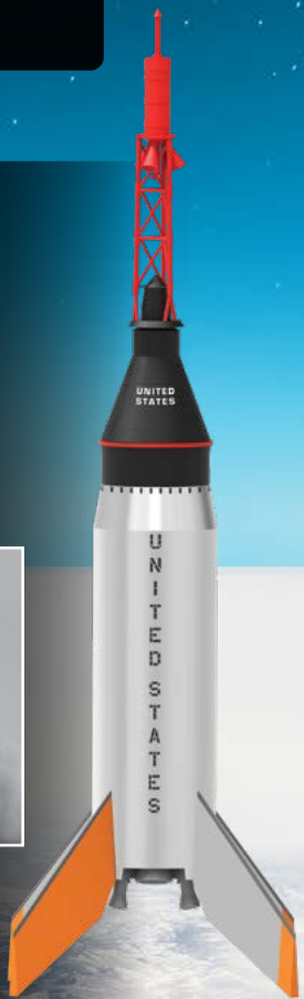
The Little Joe I booster was the first rocket designed solely for manned spacecraft qualifications and to measure critical parameters in flight.
