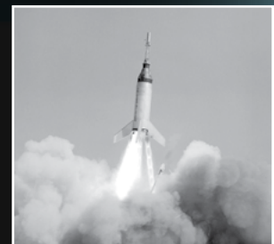
The Little Joe I booster was the first rocket designed solely for manned spacecraft qualifications and to measure critical parameters in flight.
