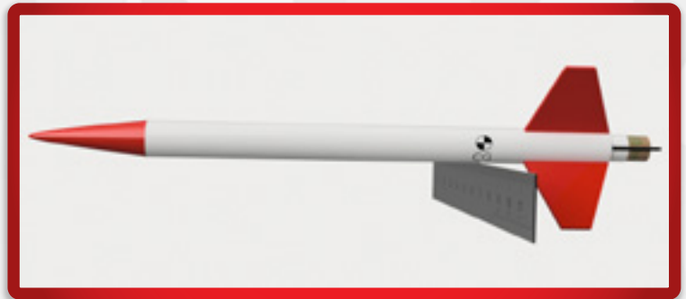
FIGURE 2 - TO FIND THE CG, YOU SIMPLY BALANCE THE ROCKET ON A RULER'S EDGE.
