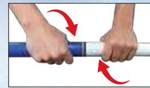
**Twist the 2 halves of the Mean Machine body tube in opposite directions and then pull apart.**
