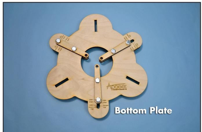
7.) Install the three legs to the lower base plate. **DO NOT GLUE THEM!** They are installed by slipping the slotted tab into the slot on the base plate. The slotted tab of the leg will be fully visible on the top side of the base plate. Now slide one of the leg lock-down keys through the slot. It should fit snugly and hold the leg firmly to the base plate.
